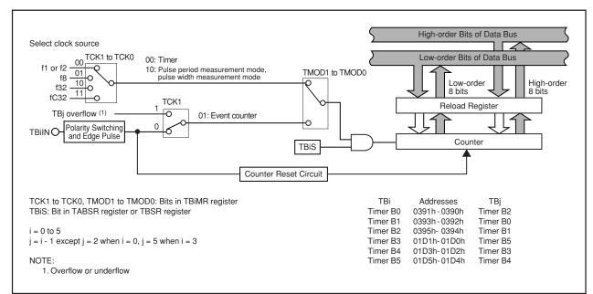
Figure 12.15 Timer B Block Diagram
